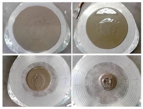
Fig. 1. Slump tests of cement pastes, W/C = 0.65, 0.60, 0.45, 0.35
